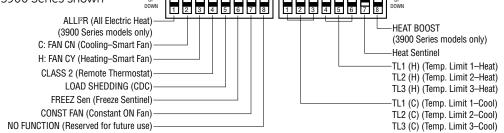
Cooling and Heating temperature limits are set independently, temperature limiting switches are in factory-set down position, except as noted.
